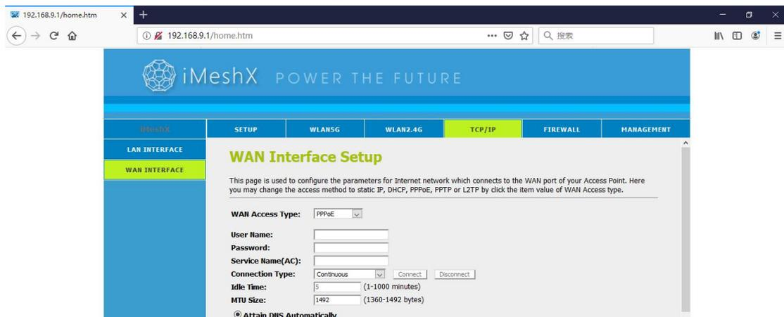
e. Connect to the Probe S WiFi network using the default WiFi network name (SSID) iMeshX-xxxxxx-2G or iMeshX-xxxxxx-5G and password on the principal gateway mine label. (for security reasons, users can modify the WiFi name and password later according to the system background feature prompt or mobile phone APP custom modification.).
